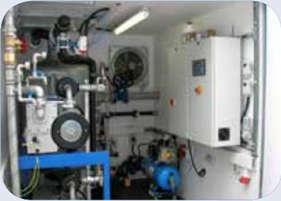
Multiphase extraction system housed in a container with noise-abatement features
